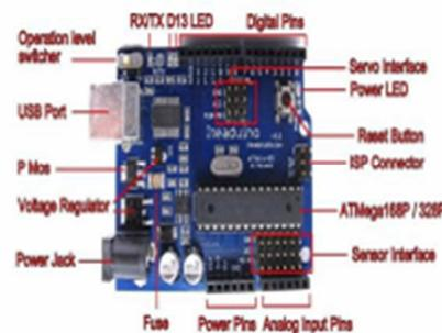
Figure 3 Arduino Board Description
