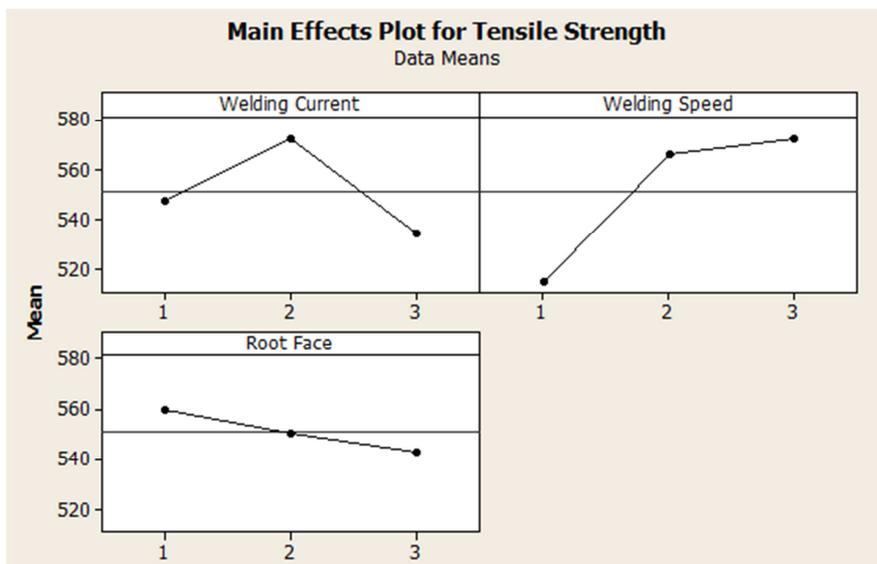
Figure 2 – Main Effects Plot for Tensile Strength
