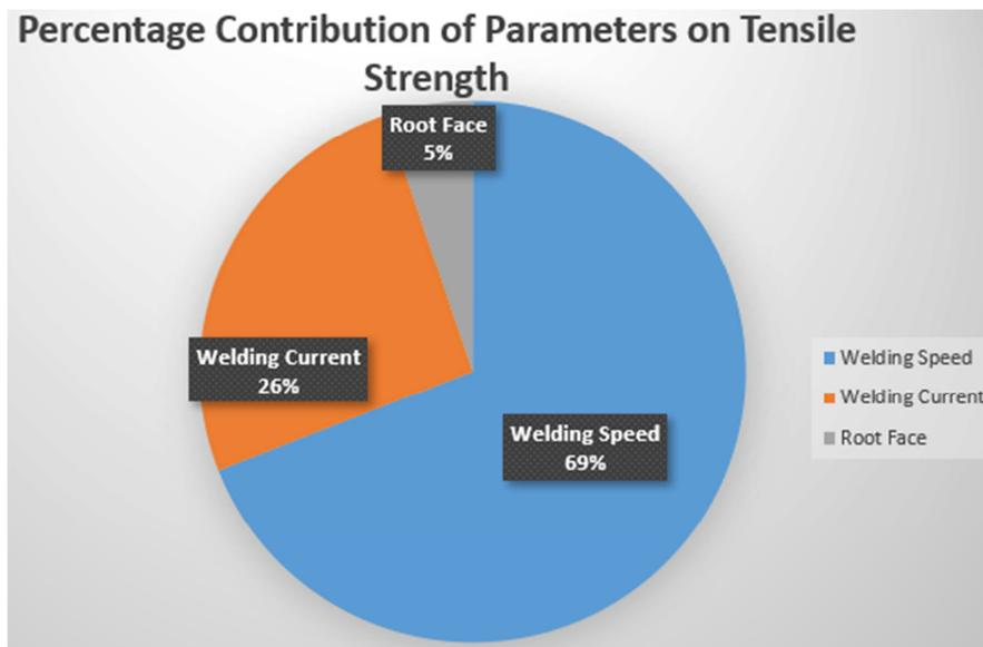
Figure 3 – Pie Chart of Parameters Effect on Tensile Strength
