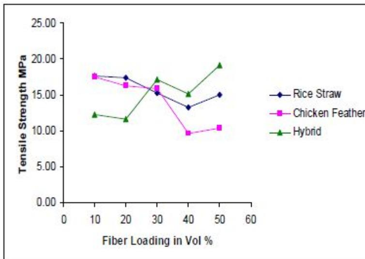
Fig. 1. Variation of Tensile Strength with Volume Proportion.
